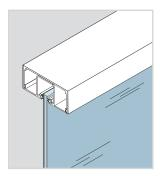
The design of the DORMA RP header system allows for a glazing pocket to be snapped into the header tube to permit a seamless transition to the sidelite glazing. The Dri-Fit gasket is used for quick and easy installation. Profiles are available for glass thicknesses of 3/8" (10 mm), 1/2" (12 mm), 5/8" (15 mm), and 3/4" (19 mm) tempered glass.
